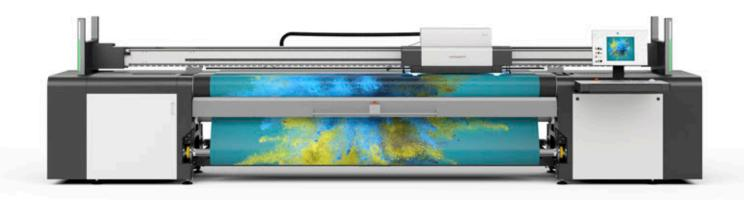
Max. productivity 212 m²/h Colours CMYK + 5 colours Max. print width 3.4 m Max. roll weight 200 kg
